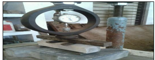
Fig 3.11 Flexural strength test on mortar beam
