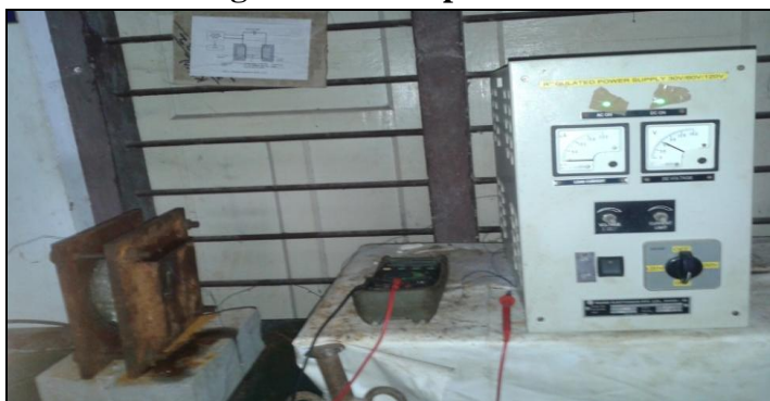
Fig 3.16 RCPT setup in the laboratory
