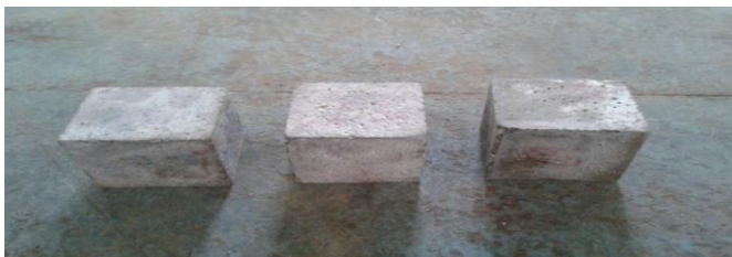
Fig 3.12 Mortar specimens subjected to sulphate attack
