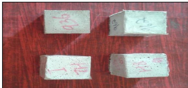
Fig 3.13 Mortar specimens subjected to acid attack
