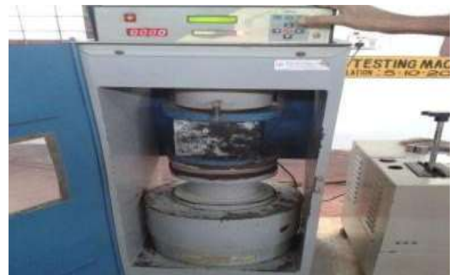
Fig.3.3 Compressive strength test on cubes
