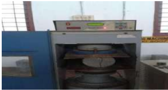
Fig. 3.4 Split Tensile strength test on cylinders
