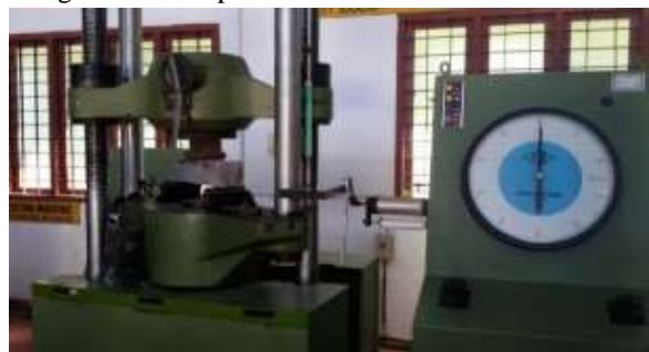
Fig. 3.5 Flexural Strength Test on Concrete Beam
