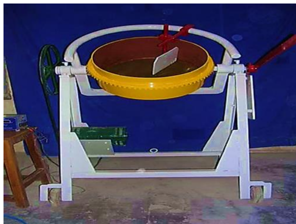
Figure 3.2 Photographic view of disc pelletizer
