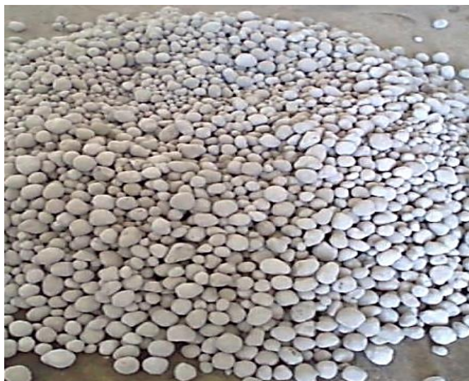
Figure 3.3 Prepared fly ash aggregates
