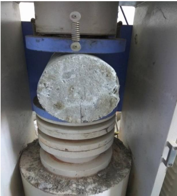
Fig. 6.3 Tensile Strength Test of Concrete
