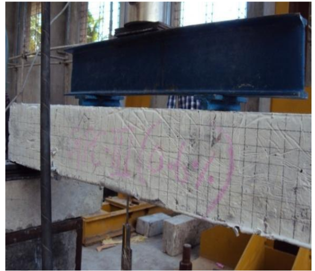
Fig. 6.7 RC Beam Test Setup
