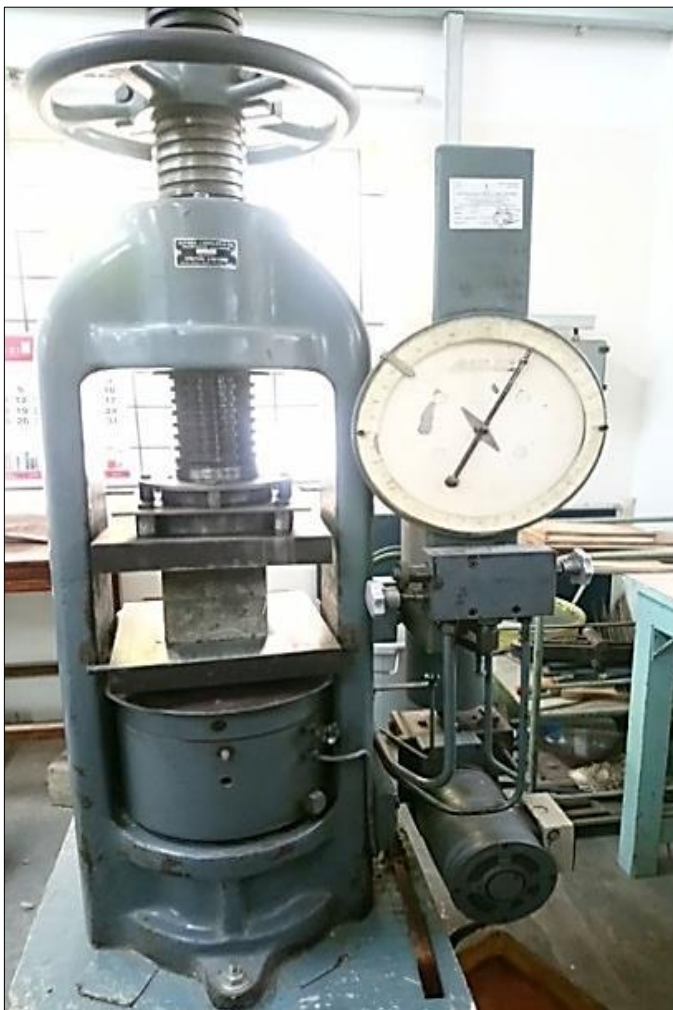
Fig.3.8 Compressive strength test setup
