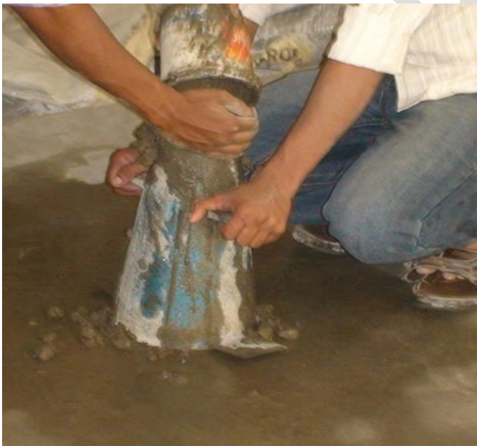
Fig. 3.3 Slump flow test
