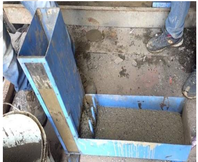
Fig.3.4 L – Box test apparatus
