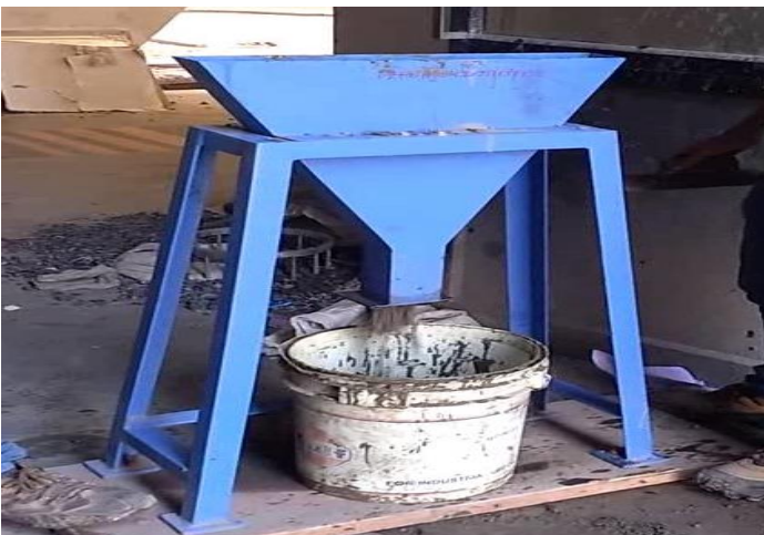
Fig.3.5 V – funnel test apparatus
