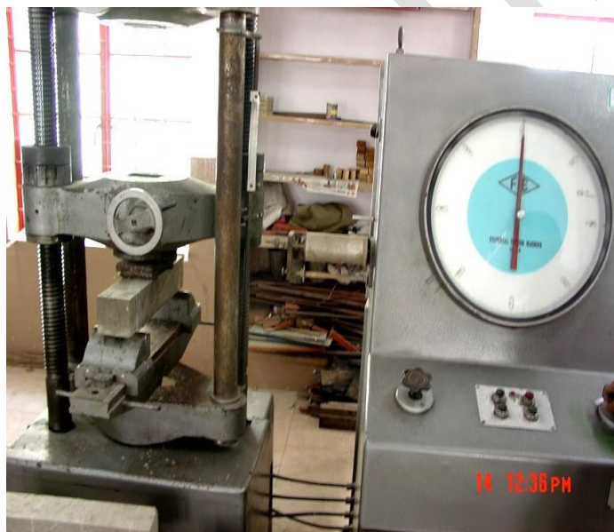
Fig.5.2 Compressive strength test setup
