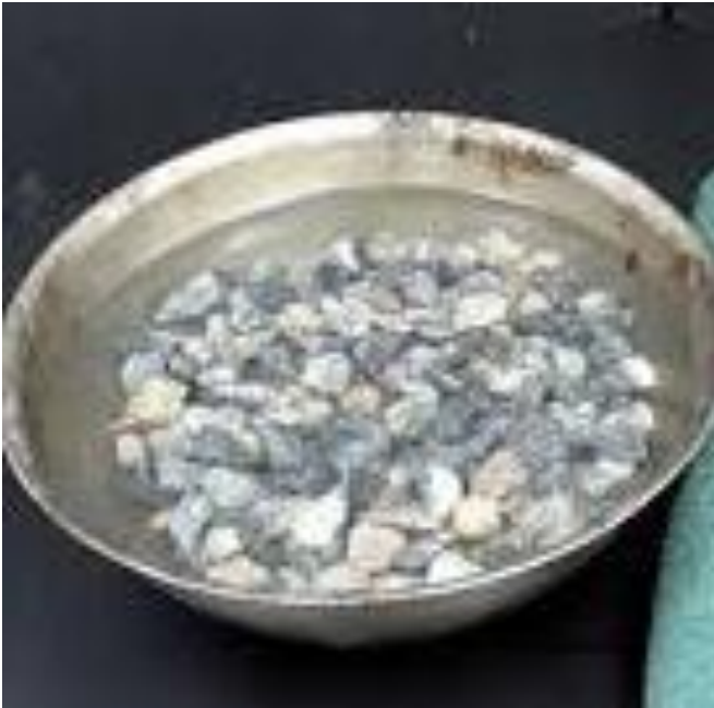
Fig 3.7 Water Absorption Water
