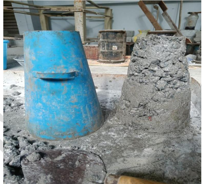
Fig6. Slump Cone Test
