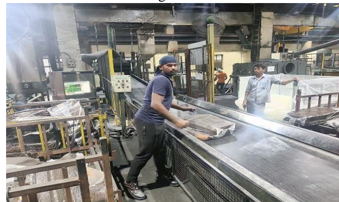
Figure: Operator again bent to drop the lifted rubber to drop into conveyor
