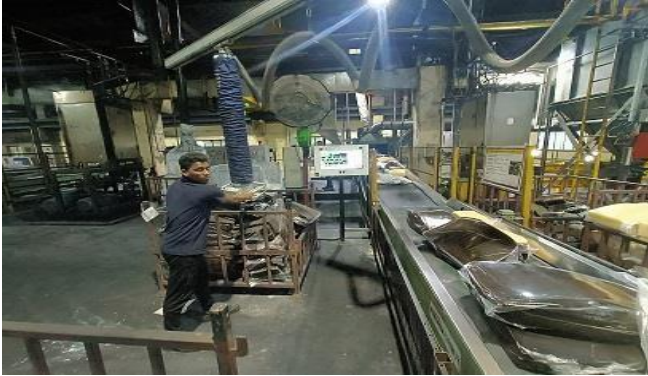
Figure: Operator lifting the rubber with the help of vacuum lifter
