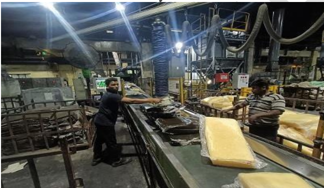
Figure: Placing of the rubber in the conveyor for the mixing process
