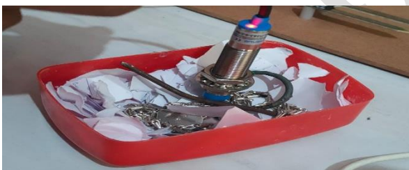
2(a) Working of proximity sensor Response
