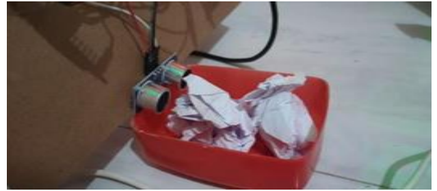
3(a) working of ultrasonic sensor when bin is filled with waste
